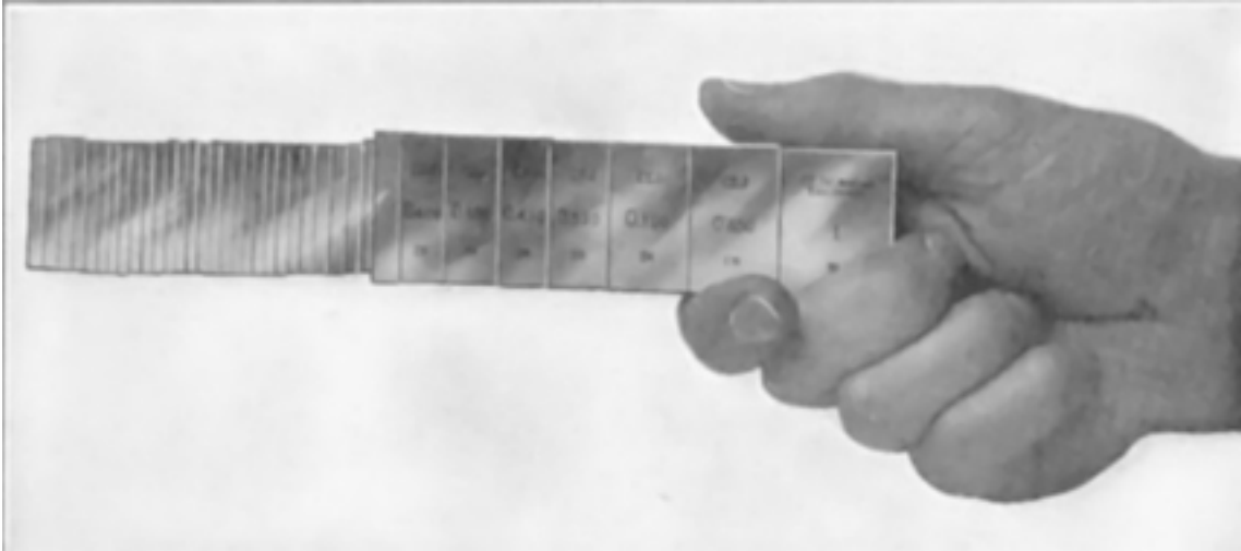
36 Johansson gauge blocks wrung together easily support their own weight
