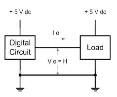
The circuit may not be capable of delivering the necessary  $I_o$  while maintaining +5 V.  $V_{OH,min}$  is the minimum value of the output voltage when high.
