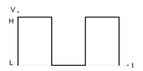
The two discrete levels are represented as low level (L) and high level (H). It is called a logic (binary) signal.
