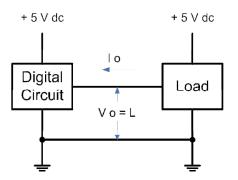
The digital circuit must act as a current sink. It must be capable of accepting a current  $I_o$  from the load and delivering to ground.  $V_{OL,max}$  is the maximum value of the output voltage when low.
