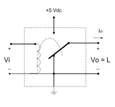
The coil current develops a magnetic field that moves the switch arm from one contact to the other. Switches and relays were useful in the construction of early machines used for calculation and/or logic operations.
