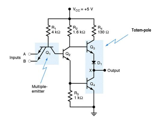
The circuit consists of multiple-emitter input transistor  $Q_1$ , phase-splitter transistor  $Q_2$ , and totem-pole transistors  $Q_3$  and  $Q_4$ .
