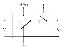
When G is low (0), this switch is open and the output is disconnected from the buffer.
